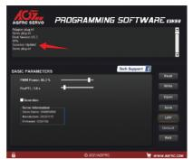
3 After finished updated the servo firmware, the servo paramater will be read automatically on the software interface.
