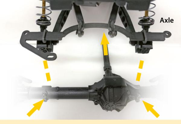
**Take the axle** with the exchanged knuckles and crawlster®4Wd-VP knuckle links **and fix them** onto the shock-absorber connectors which have been prepared with the steering system. *Remember assembling the drive shaft!*
