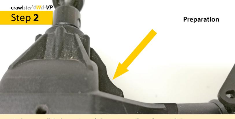
**Make a small indentation** of about 4 mm (from front right) in the central ridge of the differential housing
