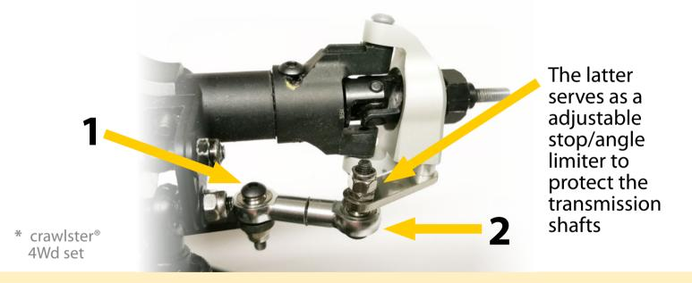
Tightly screw the **hinged brackets** with M3x15\* flathead screw from below **(1)** onto the steering bracket – lock with lock nut M3\* – and on the knuckle links with screw M3x15\* <u>from above</u> **(2)**; tighten with counternut\* <u>plus locknut</u>\* below.
