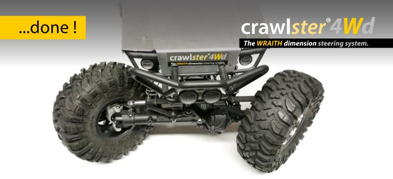
If the crawlster®4Wd steering system has been properly assembled and the transmitter is set at 100%, the wheels should have reached their limit of movement, ie. the <u>inner</u> wheel should have stopped a few mm from the front/bottom links, the <u>outer</u> wheel on the stop of the front steering arms. Slightly adjust the movement limits if necessary.
